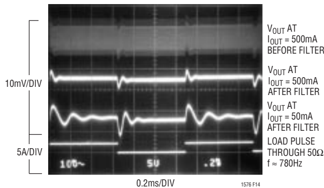
Figure 14. Loop Stability Check
