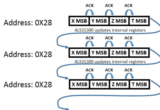
Figure 7: Fast Loop Mode
