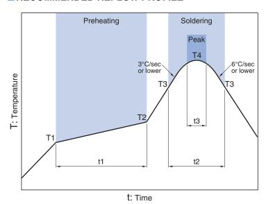
Soldering Preheating Critical zone (T3 to T4) Peak Temp. Time Temp. Time Temp. Time T1 T2 ТЗ T4 t3\* t1 t2 150°C 200°C 60 to 120sec 217°C 60 to 120sec 240 to 260°C 30sec max.
