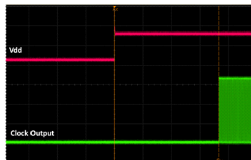
Figure 17. Startup Waveform vs. Vdd
