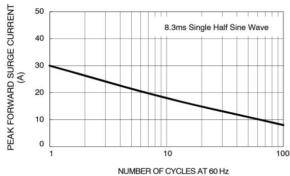
Figure 3. Maximum Non-Repetitive Forward Surge Current
