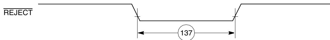
Figure 63. CAM Interface \overline{\text{REJECT}} Timing Diagram
