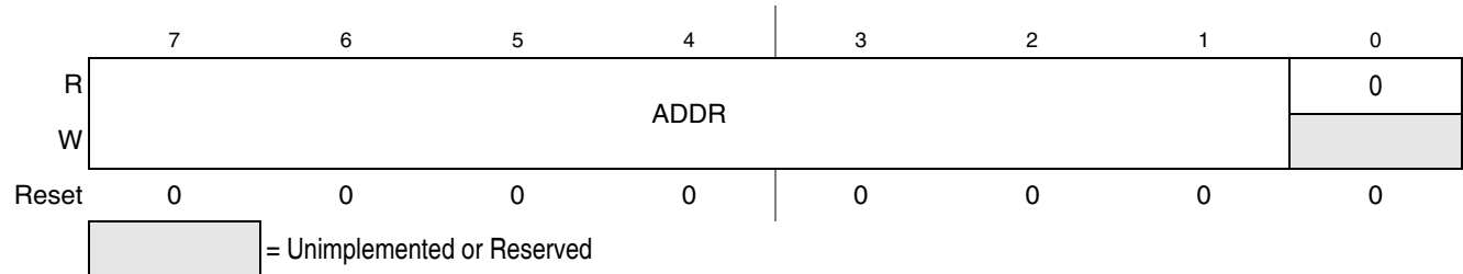
Figure 13-3. IIC Address Register (IIC1A)
