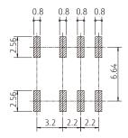
PC board mounting pad layout (TOP VIEW)
