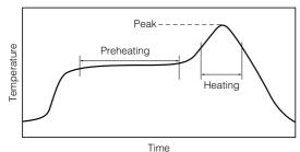
For soldering (Example : Sn/Pb)
