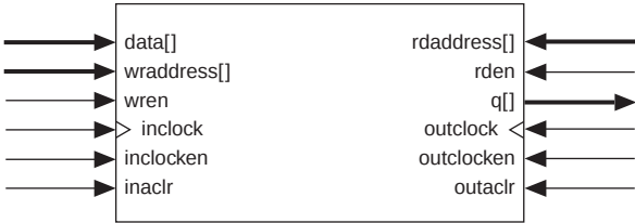
Figure 2–13. Simple Dual-Port & Single-Port Memory Configurations
