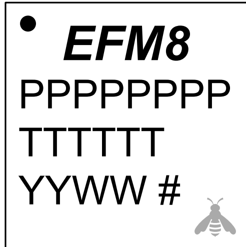
Figure 9.3. QFN32 Package Marking
