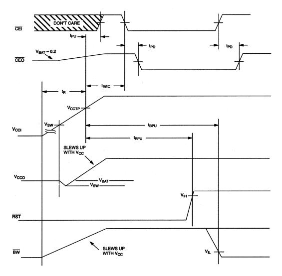
**NOTE:** If  $V_{BAT} < V_{SW}$ ,  $V_{CCO}$  will begin to slew with  $V_{CCI}$  when  $V_{CCI} = V_{BAT}$ .
