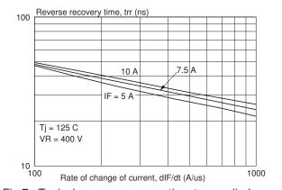
Fig.7. Typical reverse recovery time t<sub>rr</sub>, per diode as a function of rate of change of current dl<sub>F</sub>/dt.
