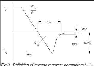
Fig.9. Definition of reverse recovery parameters  $t_{rr}$ ,  $l_{rrm}$
