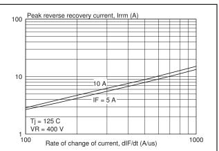
Fig.8. Typical peak reverse recovery current per diode,  $I_{rrm}$  as a function of rate of change of current  $dI_{r}/dt$ .
