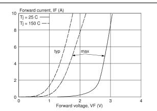
Fig.12. Typical and maximum forward characteristic per diode,  $I_F = f(V_F)$ ;  $T_i = 25^{\circ}C$  and  $150^{\circ}C$ .
