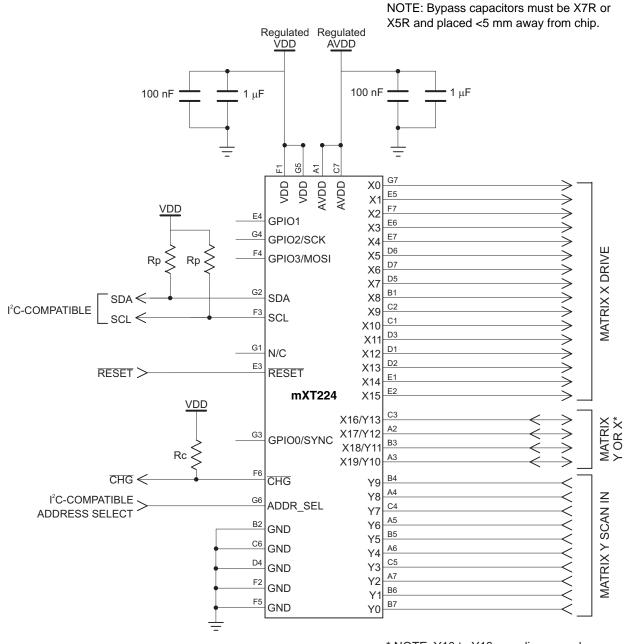
\* NOTE: Y10 to Y13 scan lines may be used as additional X drive lines in extended mode (a  $100\Omega$  resistor must be added to each additional line).
