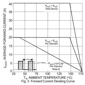
Note: 6. Black Aluminium Heatsink; length 37mm, width 15mm, height 50mm.
