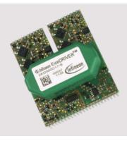
EiceDRIVER<sup>™</sup> – Gate Driver ICs and boards Highly reliable solutions for driving MOSFETs, IGBTs and IGBT modules which enable our customers to build reliable and efficient applications.
