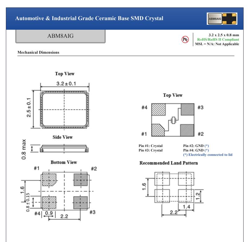
**Note:** Due to availability of raw materials, this part may be manufactured with the chamfer on pin 1 or pin 4. Be advised that this does not affect the electrical characteristics of the crystal in any way.
