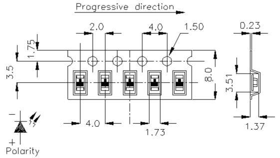
**Note:** The tolerances unless mentioned are  $\pm 0.1$ , unit=mm.
