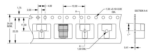
TOLERANCES: ±0.13 UNLESS OTHERWISE SPECIFIED DIMENSIONS: MILLIMETERS
