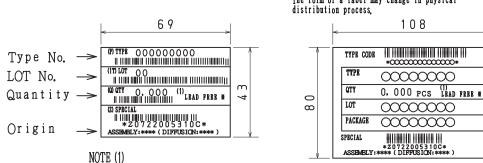
The LEAD FREE \* description shows that the surface treatment of the terminal is lead free.
