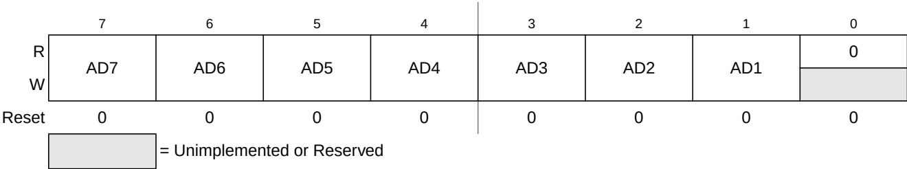
Figure 10-3. IIC Address Register (IICA)
