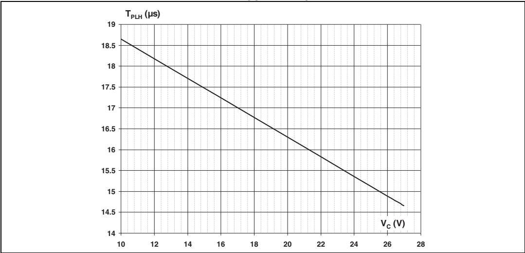
Figure 6. Variation of the input-output propagation delay time T_{PLH} at rising edge versus the supply voltage V_{CC} with R_C = 2.2\text{ k}\Omega
