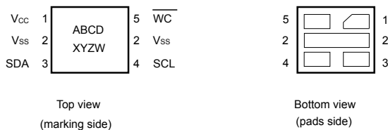
Figure 3. UDFPN5 (DFN5) package connections
