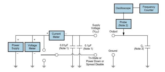
Note 1: An external 0.01µF ceramic bypass capacitor in parallel with a 0.1µF high frequency ceramic bypass capacitor close (less
