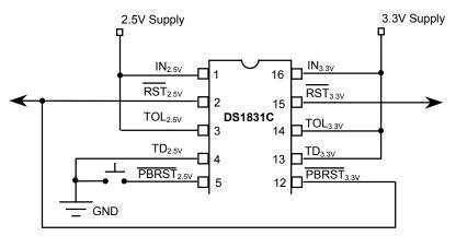
NOTE: The  $\overline{\text{RST}}_{2.5}$  volt output is connected to the  $\text{IN}_{3.3V}$  via a 100k $\Omega$  resistor in the pushbutton input and therefore does not require a pull-up resistor (an addition pull up can be used to accelerate responses.) If an external pull-up is used in this example it must be connected to the 3.3V power supply.
