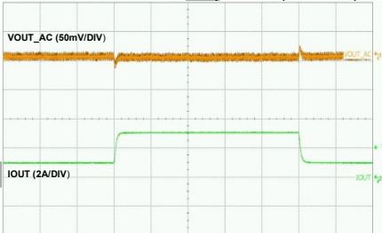
Load Transient Response (1 to 3A)
