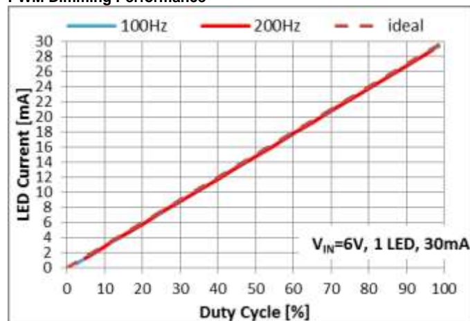
Figure 8 PWM Dimming 30mA vs. Duty Cycle
