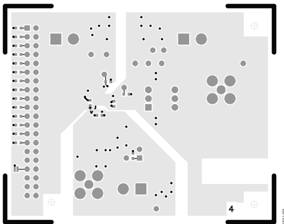
Figure 36. Evaluation Board Layout—Secondary Side
