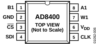
Figure 6. AD8400 Pin Configuration
