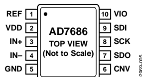
Figure 5. 10-Lead MSOP Pin Configuration
