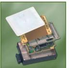
Tyco Electronics is a world leading supplier of radar technology for the automotive industries. In cooperation with system integrators and OEMs, Tyco Electronics developed 24 GHz high resolution short range radar sensors in Ultra Wide Band technology and 77 GHz Adaptive Cruise Control radar front ends suitable for driver assistance applications, which enable advanced active and passive safety systems.
