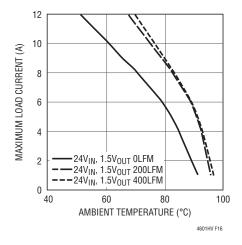
Figure 16. 24V<sub>IN</sub>, 1.5V<sub>OUT</sub>, BGA Heat Sink
