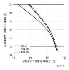
Figure 13.  $12V_{IN}$ ,  $3.3V_{OUT}$ , No Heat Sink
