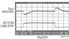
2.5V AT 6A/µs LOAD STEP C<sub>OUT</sub> = 3 • 22µF 6.3V CERAMICS 470µF 4V SANYO POSCAP C3 = 100pF
