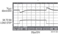
1.8V AT 6A/µs LOAD STEP C<sub>OUT</sub> = 3 • 22µF 6.3V CERAMICS 470µF 4V SANYO POSCAP C3 = 100pF
