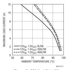
Figure 12. BGA Heat Sink 12V<sub>IN</sub>
