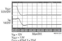
$V_{OUT} = 1.5V$   $C_{OUT} = 470 \mu \text{F}, 3 \times 22 \mu \text{F}$  SOFT-START = 10 nF
