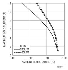
Figure 14. 12V<sub>IN</sub>, 3.3V<sub>OUT</sub>, BGA Heat Sink
