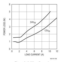
Figure 8. 3.3V<sub>OUT</sub> Power Loss
