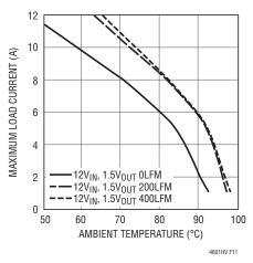
Figure 11. No Heat Sink 12V<sub>IN</sub>
