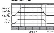
$V_{IN} = 12V$ V<sub>OUT</sub> = 1.5V C<sub>OUT</sub> = 470μF, 3 × 22μF SOFT-START = 10nF
