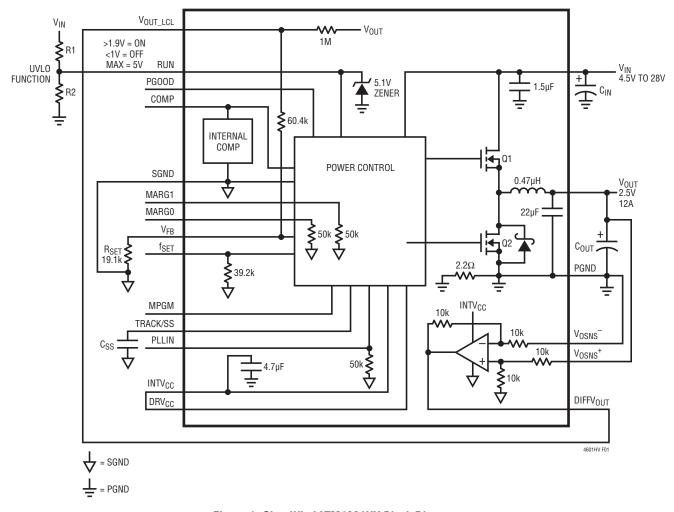
Figure 1. Simplified LTM4601HV Block Diagram
