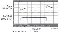
1.2V AT 6A/µs LOAD STEP C<sub>OUT</sub> = 3 • 22µF 6.3V CERAMICS 470µF 4V SANYO POSCAP C3 = 100pF
