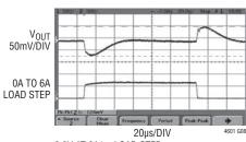
3.3V AT 6A/µs LOAD STEP C<sub>OUT</sub> = 3 • 22µF 6.3V CERAMICS 470µF 4V SANYO POSCAP C3 = 100pF
