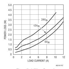
Figure 7. 1.5V<sub>OUT</sub> Power Loss
