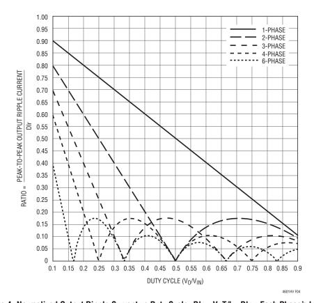
Figure 4. Normalized Output Ripple Current vs Duty Cycle,  $DIr = V_0T/L_1$ , DIr = Each Phase's Inductor Current
