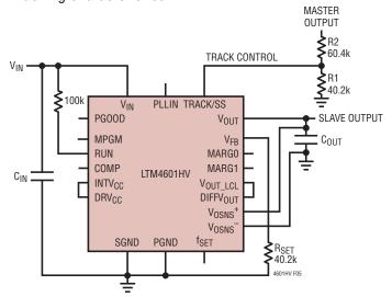
Figure 5. Coincident Tracking Schematic
