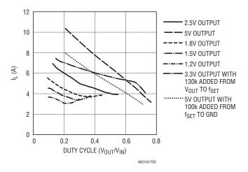
Figure 3. Inductor Ripple Current vs Duty Cycle
