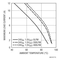
Figure 15.  $24V_{IN}$ ,  $1.5V_{OUT}$ , No Heat Sink
