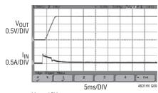
V<sub>IN</sub> = 12V V<sub>OUT</sub> = 1.5V C<sub>OUT</sub> = 470µF, 3 × 22µF SOFT-START = 10nF
