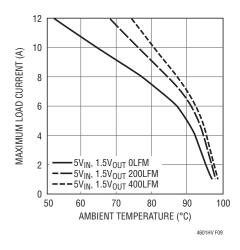
Figure 9. No Heat Sink 5V<sub>IN</sub>
