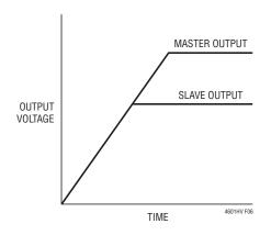
Figure 6. Coincident Output Tracking Characteristics
