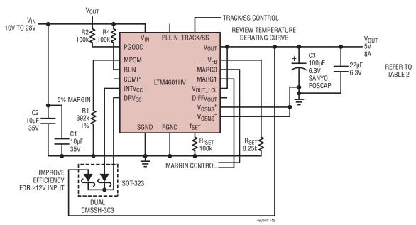
Figure 18. 5V at 8A Design Without Differential Amplifier
