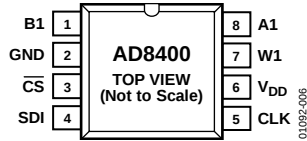
Figure 6. AD8400 Pin Configuration
