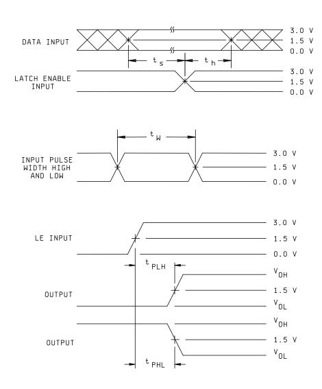
FIGURE 4. Switching waveforms and test circuit.
