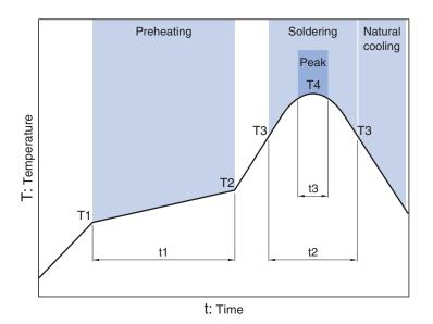
Preheating Soldering Peak Temp. Temp. Time Time Temp. Time Τ1 T2 **T**4 t1 тз t2 t3 150°C 180°C 60 to 120s 230°C 260°C 10s 30s
