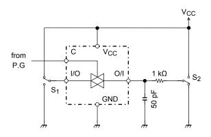
2. Cross Talk (control input-switch output) flN = 1 MHz duty = 50% tr = tf = 6 ns
