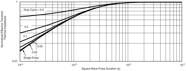
Normalized Thermal Transient Impedance, Junction-to-Foot
