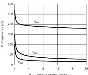
$V_{DS}$  - Drain-to-Source Voltage (V)  $\label{eq:capacitance}$
