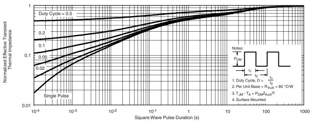
Normalized Thermal Transient Impedance, Junction-to-Ambient
