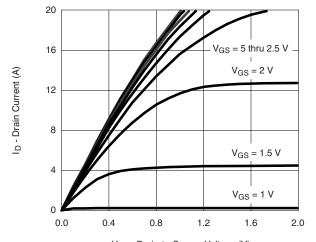
V<sub>DS</sub> - Drain-to-Source Voltage (V)
