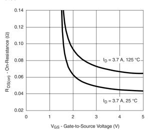
On-Resistance vs. Gate-to-Source Voltage
