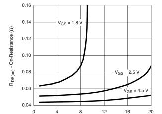
$\label{eq:loss_problem} I_D \text{ - Drain Current (A)}$  On-Resistance vs. Drain Current and Gate Voltage
