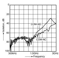
1.-(2) High frequency characteristics (Impedance 50Ω) Sample: RK1-5V
