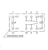
PC board mounting hole layout (BOTTOM VIEW)
