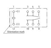
PC board mounting hole layout (BOTTOM VIEW)
