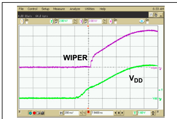
FIGURE 2-52: 50 k \Omega – Power-Up Wiper Response Time.
