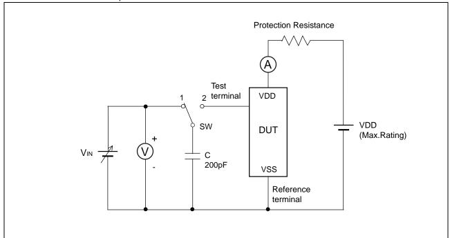
Note: Charge voltage alternately switching 1 and 2 approximately 2 sec interval. This switching process is considered as one cycle. Repeat this process 5 times. However, if the latch-up condition occurs before completing 5times, this test must be stopped immediately.
