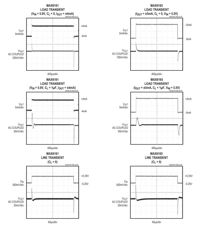
Note 5: Many of the *Typical Operating Characteristics* of the MAX6161 family are extremely similar. The extremes of these characteristics are found in the MAX6161 (1.25V output) and the MAX6165 (5.0V output). The *Typical Operating Characteristics* of the remainder of the MAX6161 family typically lie between these two extremes and can be estimated based on their output voltages.
