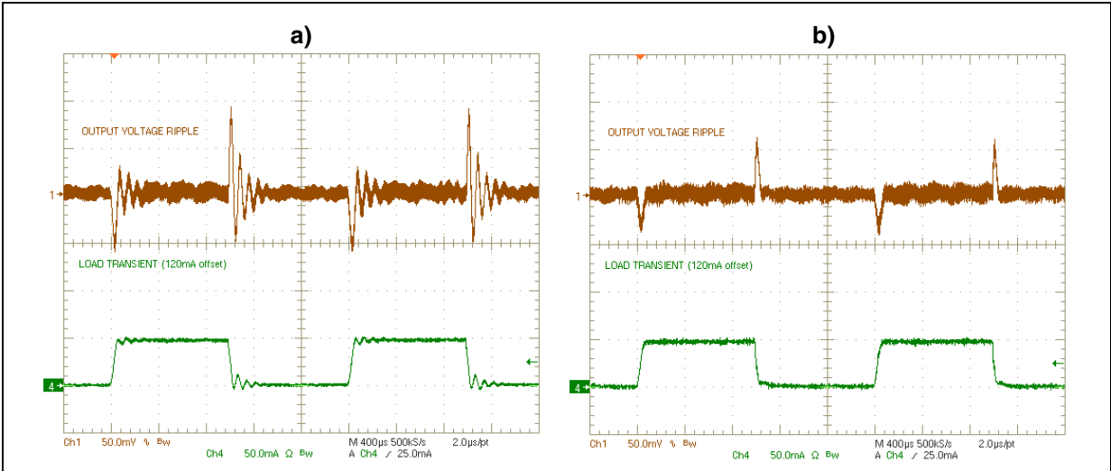
Figure 17. Poor phase margin (a) and properly damped (b) load transient responses
