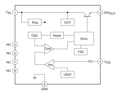
Note: Since the NC pins are not connected within the IC package, they can be used as connection points.
