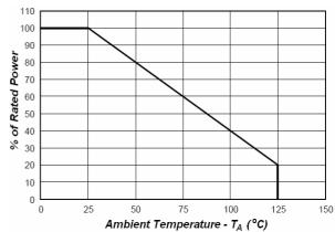
Fig2. Power Derating Curve
