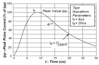
Fig1. Pulse Waveform
