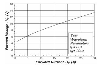
Fig3. Forward Voltage vs.Forward Current
