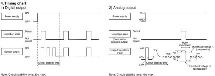
While the circuitry is stabilizing after the power is turned on, the sensor output is not fixed in the "on" state or "off" state. This is true regardless of whether or not the sensor has detected anything. Note: Circuit stability time: 45s max. While the circuitry is stabilizing after the power is turned on, the sensor output is pat fixed in the "par" citate or "inf" ctate. This is true regardless of whether or
