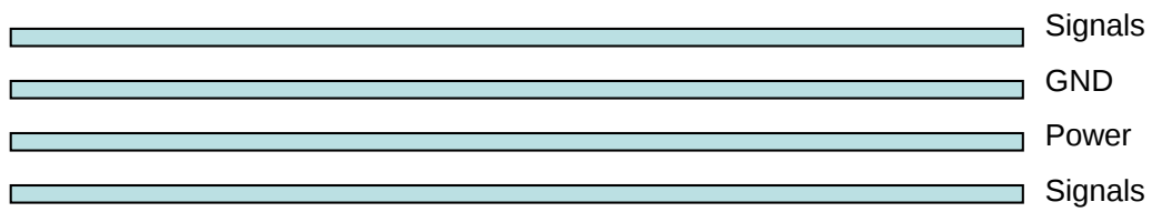
Figure 12: Typical 4-layer PCB construction
