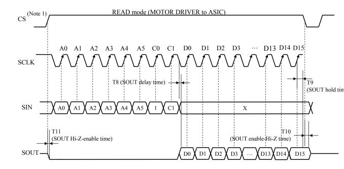
Note 1) CS default value of each cycle (Write / Read mode) starts from Low-level.
