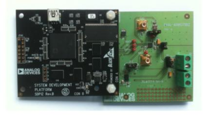
The **EVAL-AD9837SDZ** evaluation board is designed to help customers quickly prototype new AD9837 circuits and reduce design time. A high performance, on-board 16 MHz trimmed general oscillator is available to use as the master clock for the AD9837 system. Various links and SMB connectors are also available on the EVAL-AD9837SDZ board to maximize usability.
