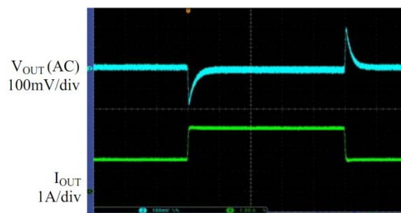
Time 200μs/div Fig. 11: Load transient I_{OUT}=1.5A to 3A
